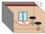
Figure 2: Three walls and angled roof. Note: in all cases, less restrictive consideration may be given if the roof is angled or pitched upwards.
